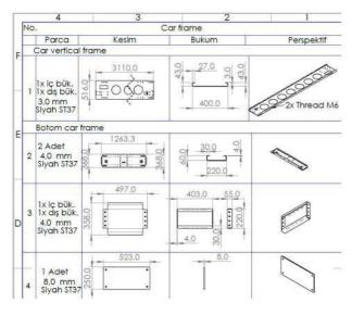
• Upon customer's confirmation, we automatically do production drawings using formulas in SolidWorks 3D Cad software. This process allows us to produce our customers' ordered goods free of defects and minimize the likelihood of our customers' encountering an unexpected problem in the elevator field.
